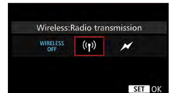
Figure 13.16 Select radio wireless and then press the Set button.
