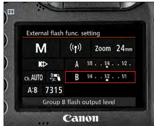
Figure 13.12 The 600EX-RT can display radio wireless settings on the LCD of 2012-and-newer camera models.
