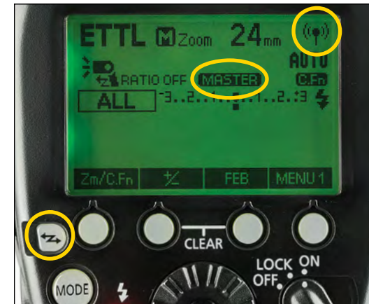
Figure 13.14 Activating the 600EX-RT as a radio master.
